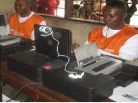
*The DRC registration kit comprises a small handheld computer, a webcam and a printer.*
