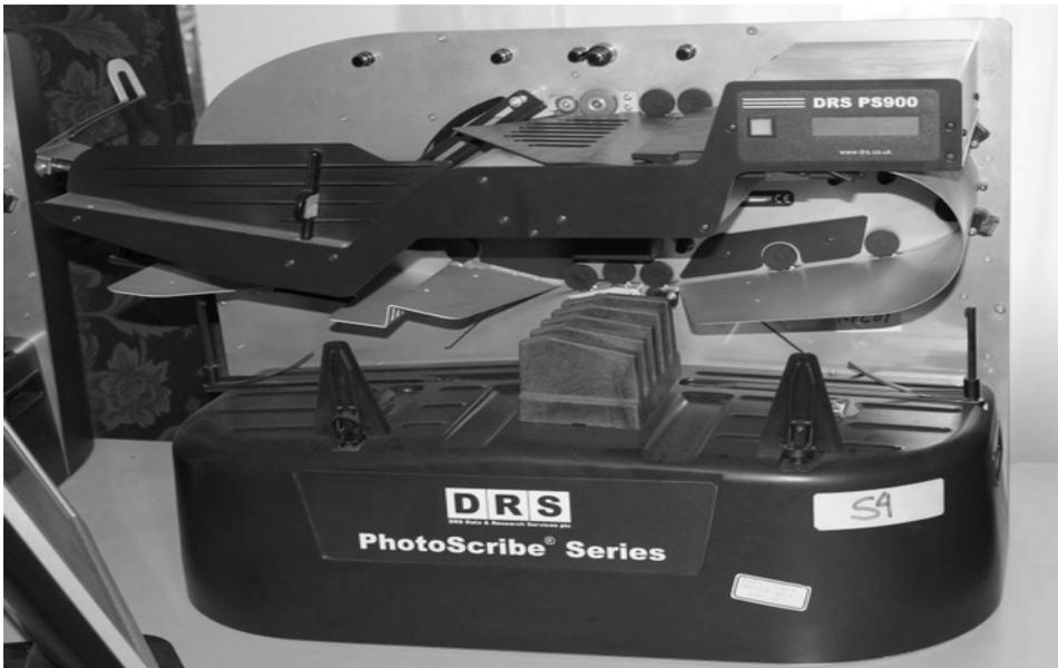
*The scanner uses combined OMR and image recognition technology. It can detect and record – in real time – a variety of items on a form including the barcode and photograph.*
