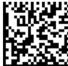
*The latest development in barcoding, called Semacode, can be read using mobile phones with built-in cameras.*
