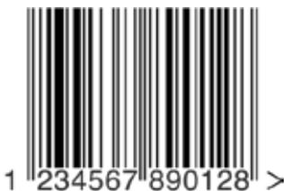
*Example of a traditional barcode: A conventional barcode reader sends a laser light to the barcode and measures the light that is reflected back.*
