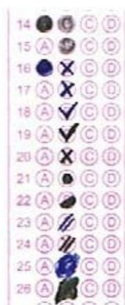
*A completed OMR form: The scanner software can identify number 14 as 'A', number 15 as 'B', number 16 as 'A' and numbers 17 to 26 as 'B'. Some of the boxes have been marked using blue or black pen and pencil, but modern technology can still read the markings correctly.*
