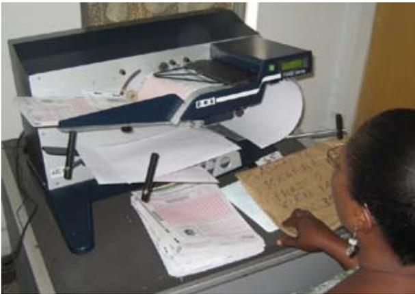
*Despite the fact that vendors quote a higher rate, the practical experience of Ghana is that the scanners can process about 1,000 forms an hour in real working conditions.*
