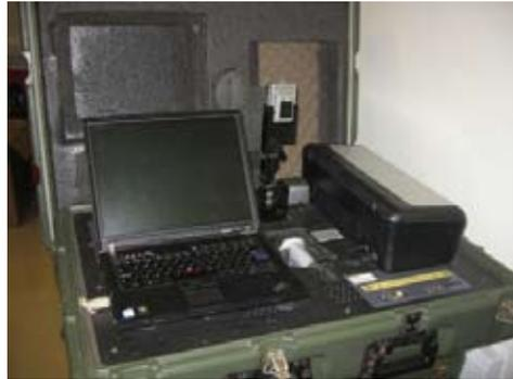
*The second generation registration kit used in Ghana comprises a computer, a digital camera and a printer. The first generation kit used a Polaroid camera.*
